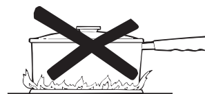
These flames are too large for the pot
