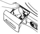
Do not exceed the maximum fill line. Overfilling can cause early dispensing of the bleach which could result in damaged clothes.
