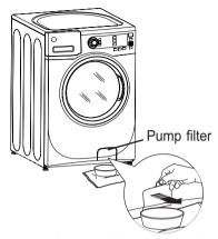
Using a coin or flat screwdriver in the notch on the door, open the access door.
