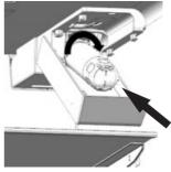
4. Push the filter, and then turn it clockwise until it locks. If you have trouble inserting the water filter because of high water pressure, shut off the water supply valve
