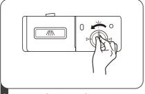
1 Remove the rinse aid reservoir cap by rotating it counterclockwise.
