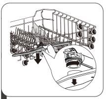
To remove the upper spray arm, hold the nut in the center still and rotate the spray arm counterclockwise to remove it.
