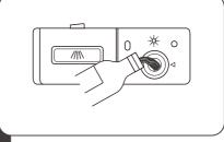
Carefully pour in the rinse-aid into its dispenser, whilst avoiding it to overflow.
