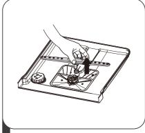
To remove the lower spray arm, pull out the spray arm upward.
