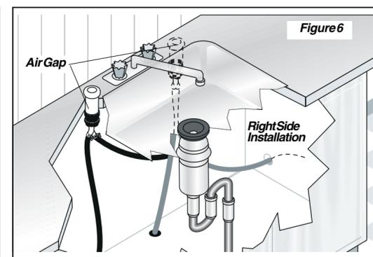
3. If you connect to a sink trap, local codes may require you to install an air gap kit, (not included). The drain hose will be routed from dishwasher to air gap inlet as shown in Figure 6. An air gap kit is available from a plumbing supply store. NOTE: If the drain hose is installed through the floor, an air gap is necessary.
