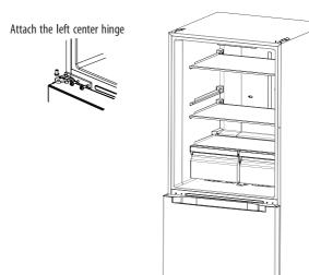
7)Put down the refrigerate door on the middle hinge vertically, then take out the top hinge and cover of other side from accessory bag, assemble top hinge, hinge cover and hole cover.
