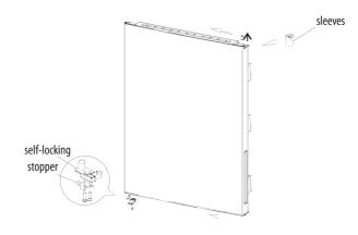
6)Remove the center hinge,removethe center hinge shaft with a slotted screwdriver, install hinge shaft on opposite side of the hinge andinstall the hinge to the left of the box.
